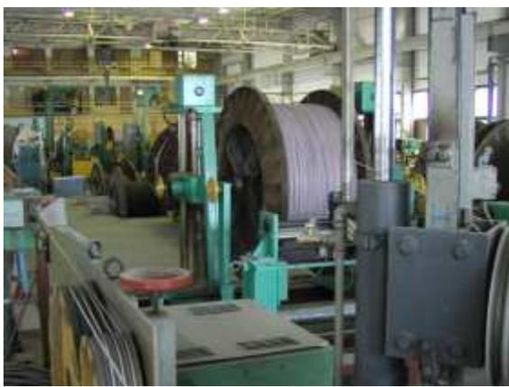
Along with traditional submersible cable (КРРР, КРрРР) (working temperature 120°C) the Company fabricates heat-resistant cable (working temperature till 230°C). There are cable with EPDM insulation and cable with EPDM and polyimide film. Cable has lead jacket. The Company fabricates cable (type КИФРР) (working temperature 230°C). Insulation is polyimide film and two extruded fluoroplast layers (type 4 МБ).
